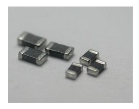
The GMPI series is magnetically shielded chip coil based on a multilayer process construction. New magnetic material was developed to get excellent direct current characteristics. There is no cross coupling between inductors due to a low magnetic shield. Lead-free and ideal for high density SMT installation with no directionality. Superior solderability and resistance to soldering heat make them ideal for wave or reflow soldering
